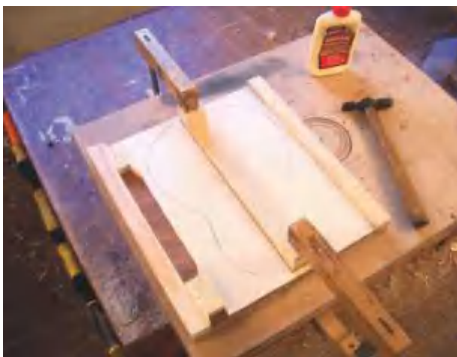
▲ Pic.32 The soundboard in the jointing jig
